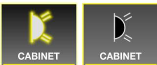
Press to cycle cabinet lights on and off. Will not function on low battery.
