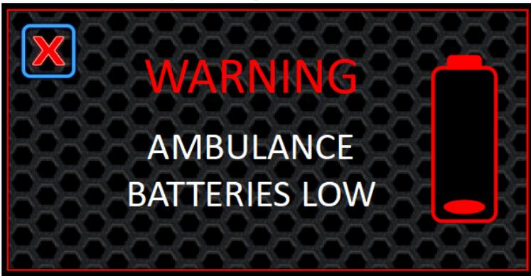
Will trigger when patient compartment battery voltage is below 11.8v. Press X at top left to dismiss. It is highly recommended you either plug in the shoreline, or run the engine to charge the batteries.
