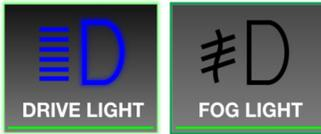
Enables the drive lights. Will run when high beams are on, and battery is not low. Will disable the fog light switch.
