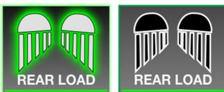
Enables the rear loading lights. Opening the rear R2 door will turn on the lights for up to 5 mins or until the door is closed. The light will remain on for 2s after the door is closed.
