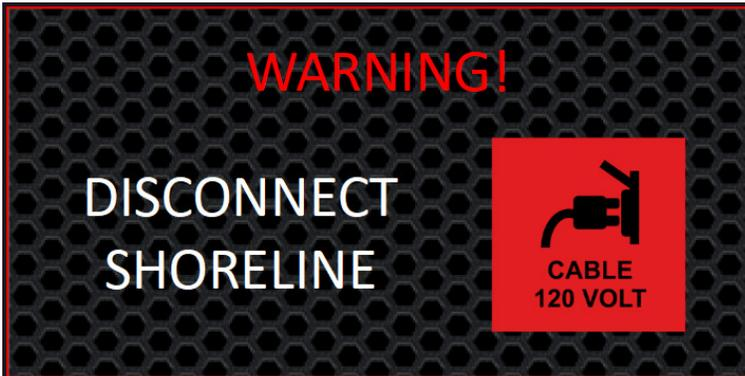
Will trigger when shoreline is connection, ignition is on, and engine is running. It will also trigger an auditory alarm. This will not trigger in the case of an auto-eject shoreline. Eject shoreline to dismiss.
