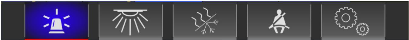
Driver SP3 pages are main(contains emergency lighting, siren, eco, and other essential controls), lighting, HVAC, seat belt monitoring and configuration. After 10 seconds of no user interaction the SP3 will revert to the main page.
