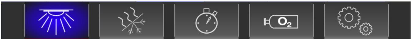
MCC SP3 pages are lighting, HVAC, timer, oxygen and configuration. The MCC SP3 has no timeout feature like the driver SP3.
