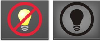
Disables the touchscreens backlight. Will automatically turn off 5 minutes after the engine and eco-run are off. Engaging the low beams will reduce the SP3 backlight for nighttime use.
