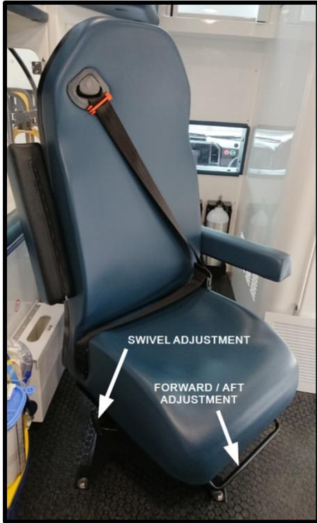
The Main (Cot head) Attendant's seat is equipped with 3-point seatbelt and forward/backward adjustable slide. It may also be equipped with a two- or eight-position swivel base. The forward/backward adjustment lever is behind the legs when sitting. The swivel lever is a pull-out style T-handle on the right-hand side of the seat.
