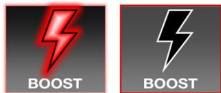
Enables the battery bypass to connect batteries for more starting power. Is automatically enabled if chassis voltage is above 13.1 volts via external battery charger or if shoreline is connected which powers onboard battery charger.
