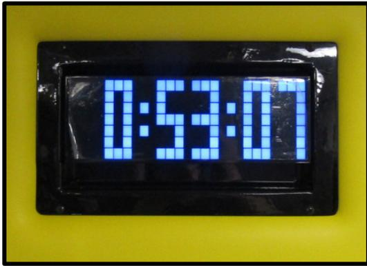
To remove the clock from its enclosure, pull the bottom out to detach the hook-and-loop strip, lift and slide off from screws in the keyholes on the back, and pull out. Be careful when pulling out the clock; electrical wires are tied to it.
