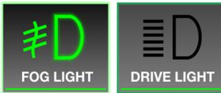
Enables the fog lights. Will run when high beams are off, and battery is not low. Will disable the drive light switch.
