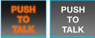
Momentary button enables the rear conversion push to talk. It will set the HVAC fans to low speed to reduce background noise.
