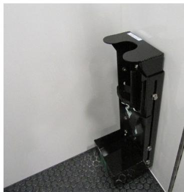
Up to four (4) portable tank brackets may be installed in the ambulance. One (1) inside patient compartment, near the front Bulkhead panel, and three (3) mounted to inside the Oxygen compartment.
