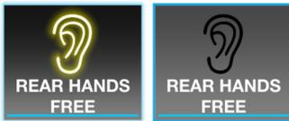
Enables the rear mic for the intercom system. Will not disable the HVAC fan like the MCC and RMCC buttons.
