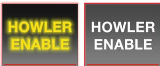
Enables the howler, can be enabled via master emergency. Pressing the chassis' horn is used to control the howler when the button is enabled.
