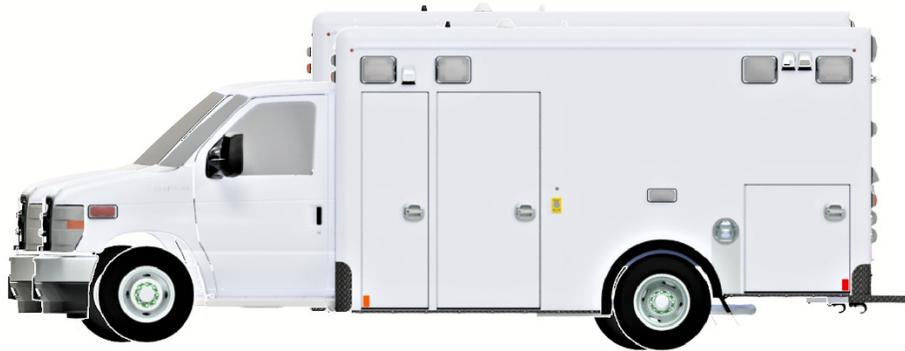
Type III – Cutaway chassis with integral patient compartment (Standard & Tall)
