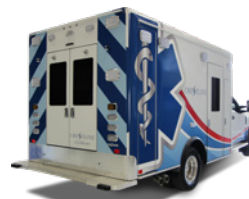
The all aluminum underbody bumper protects the module in low impact collisions.
