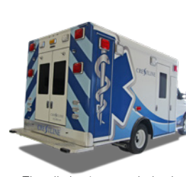
The all aluminum underbody bumper protects the module in low impact collisions.
