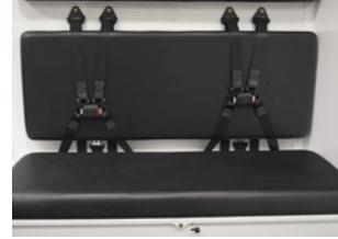
Wider Squad Bench: Improved comfort with 6" increased width
