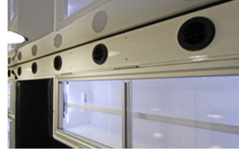
Upgraded AC Performance: 20% cooling improvement with recirculation technology and 8-speed control
