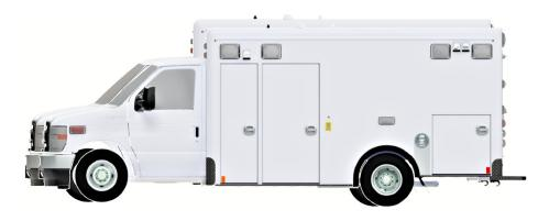
**Type III** – Cutaway chassis with integral patient compartment (Standard & Tall)
