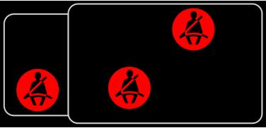
Will trigger notification and alarm when driver seatbelt, attendant (airway) seatbelt, or mobility seatbelt (if equipped) are not engaged when the seat is occupied and the vehicle is no longer in park. The Mute Button will not mute the seatbelt monitoring alarm.
