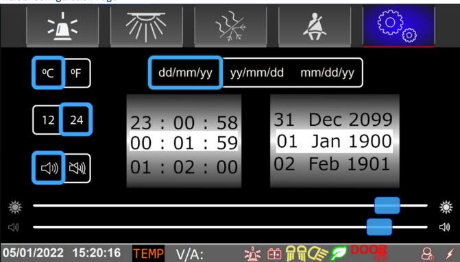
In the configuration page you can select Celsius or Fahrenheit for temperatures, 12 or 24 hour time, enable or disable the SP3 audio, the date format, the current date and time, the screen brightness, and the audio volume.
