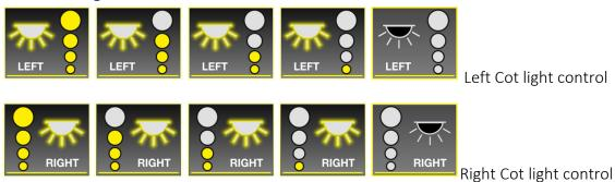
Press button to cycle through power levels. The cot lights have 4 different power levels.
